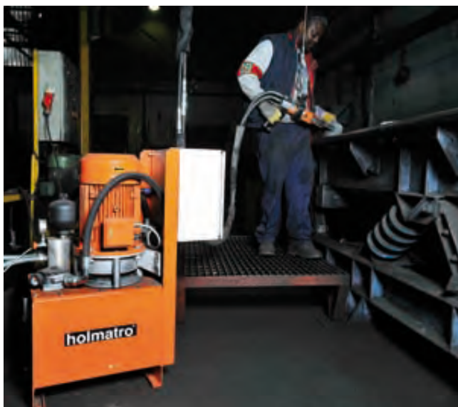
Foundry wedge fastened to crane by means of balancer
